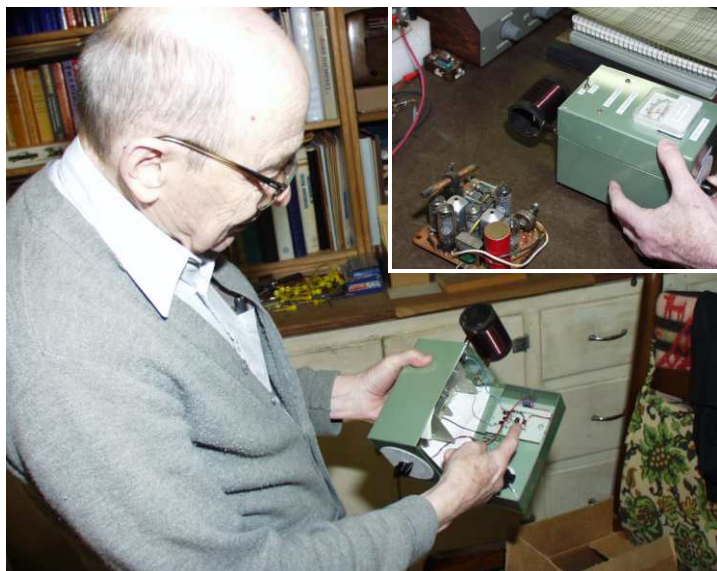
Wayne is demonstrating one of his specialized pieces of test gear. This is a Gate-Dip-Meter, but only for the broadcast band for working on old radios. In the inset it is checking the tuning of a old BC radio.
