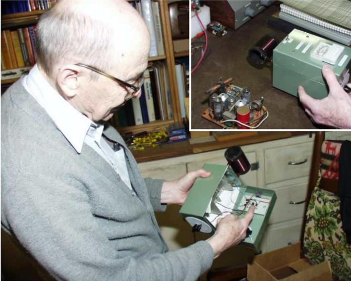
Wayne is demonstrating one of his specialized pieces of test gear. This is a Gate-Dip-Meter, but only for the broadcast band for working on old radios. In the inset it is checking the tuning of a old BC radio.
