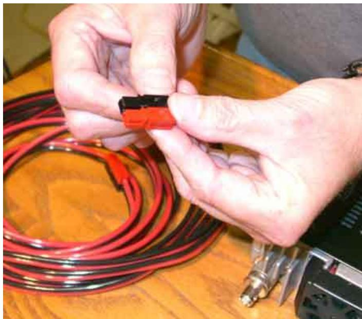
*The new Anderson PowerPole connectors which will become the standard for ARES. This insures that in emergencies all converted rigs will have the same power connectors so they will interchange quickly.*
