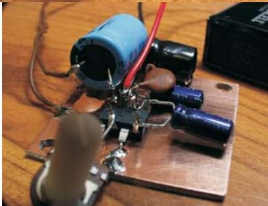
And don't forget to observe the polarity on the capacitors. When you connect them backwards they have a nasty habit of blowing up in your face after being powered up for about 10 minutes. It sounds like a firecracker. A most rude awakening, especially late at night when the little aluminum can bounces off your forehead and capacitor-fuzz gets all in your nose, eyes and ears. Don't overheat the IC pins. A good soldering iron is a great investment.
