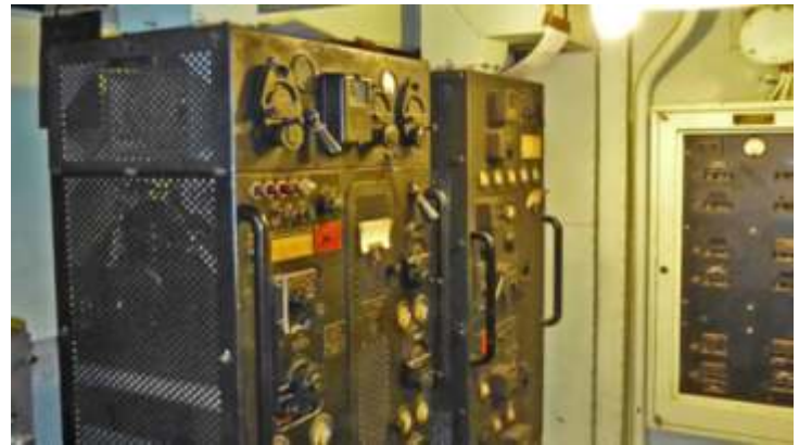
Westinghouse Model TDE transmitter, 300 - 18,100 kc, 125 watt CW, 30 watt AM phone, placed in service 9/25/44. The TDE was brought back online 5/30/2006 by "Mac" McCullough, one of the ship's original CW operators. Signal report was 579, with a hum. "But they all do that."
