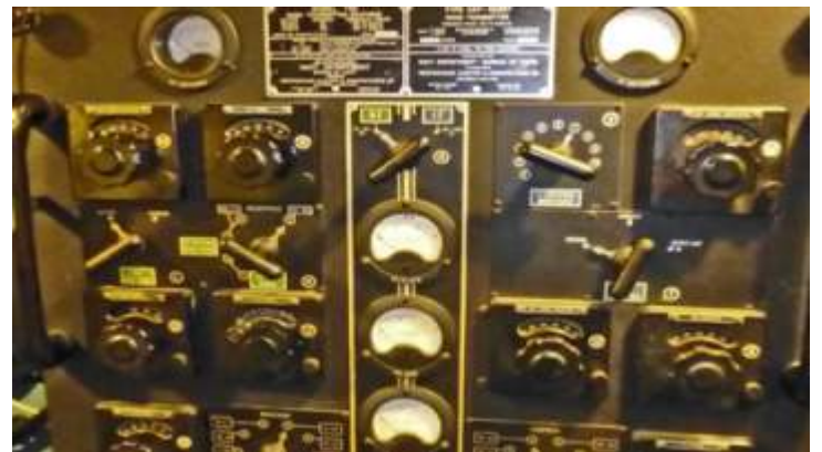
Westinghouse Model TDE transmitter, 300 - 18,100 kc, 125 watt CW, 30 watt AM phone, placed in service 9/25/44. The TDE was brought back online 5/30/2006 by "Mac" McCullough, one of the ship's original CW operators. Signal report was 579, with a hum. "But they all do that."
